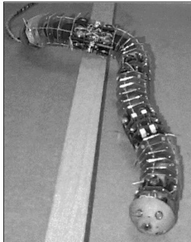
**Figure 2-17:** The GMD Snake mechanism
