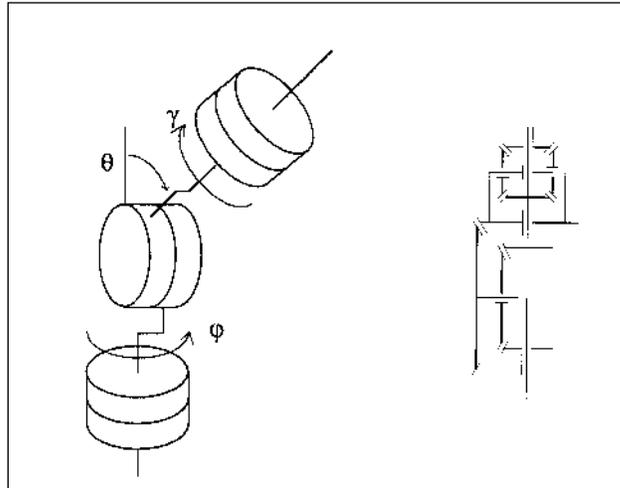
**Figure 2-15:** The PIRAIA link provides a roll-pitch-roll capability.
