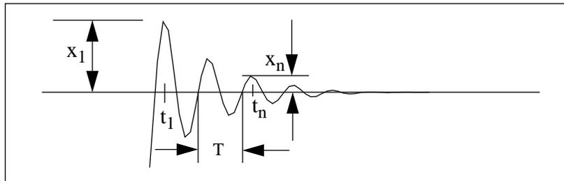
**Figure C-1:** Modeling the decaying oscillation of the servo actuator
