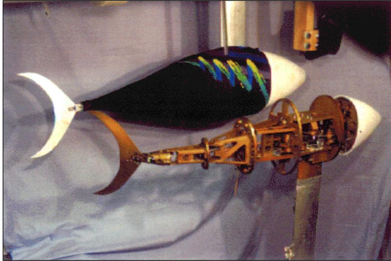
**Figure 2-21:** The RoboTuna internals and foam latex covering.
