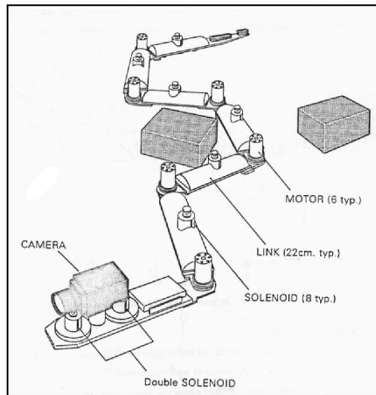
**Figure 2-12:** Shan's snake mechanism uses a concertina-like motion.
