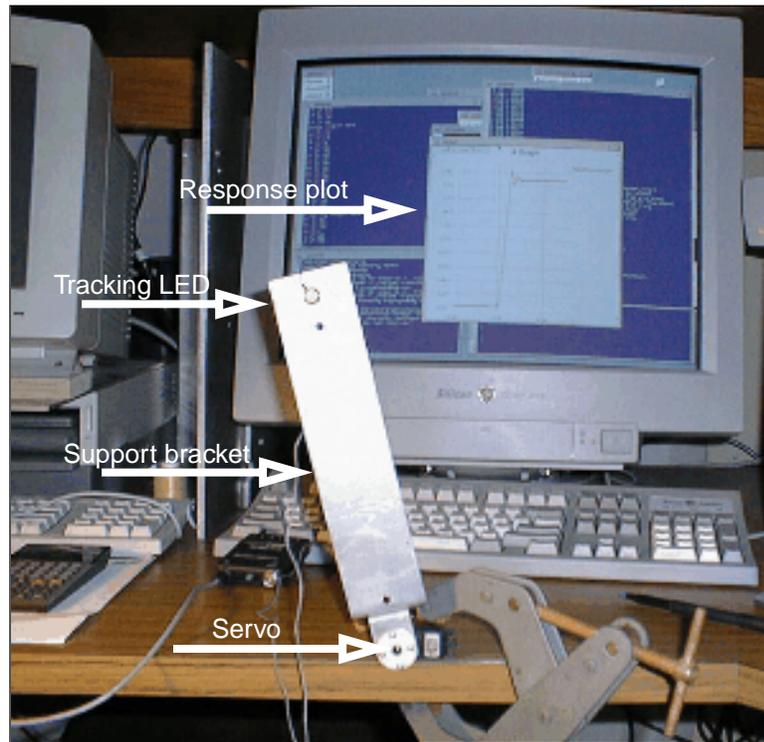
**Figure 6-3:** Test setup for determining servo model.
