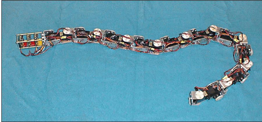
**Figure 6-11:** 3D snake utilizes 10 links with 20 servos
