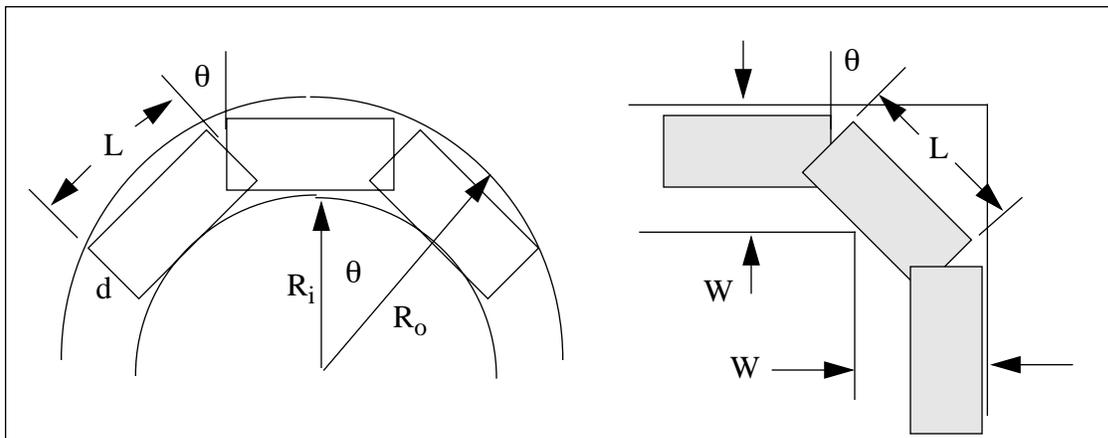
**Figure 6-5:** The relationship between link aspect ratio and joint angle motion for a right angle corridor.
