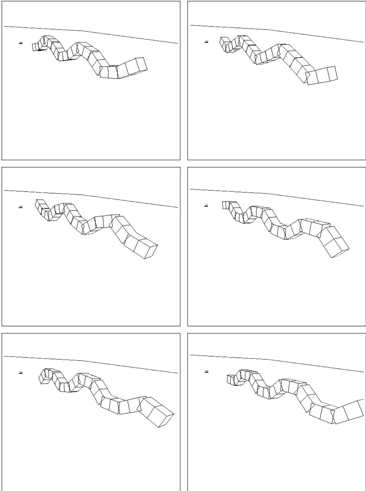
**Figure 7-4:** Rectilinear locomotion.
