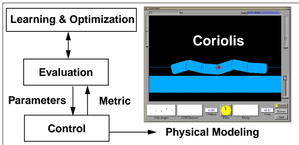
**Figure 3-1:** Framework for learning control of a physical device.
