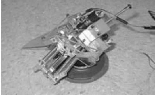
Figure 7: Photo of 2 nd Generation hopper in compressed state. The outer shell is removed for clarity.
