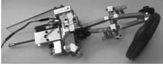
Figure 6: Side view of uncompressed 2 nd Generation hopper. The outer shell is removed for clarity.
