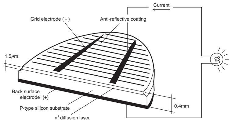
Electrons involved in forming the bonds between atoms fly out from the crystalline framework as free electrons bearing a negative charge. After the electrons have been given off, a positive electron hole is formed. An electrical field builds up inside the silicon present at the P-N junction and the electrons are scattered to the N-type silicon. A voltage is produced at both electrodes and, if a load is connected to them, electrical power is supplied to it.
